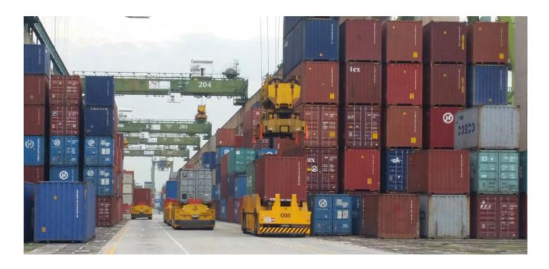
In 2040 when PSA Singapore's Tuas Mega Port is fully operational, it will be the world's largest fully automated container terminal in a single location. In preparation for this new mega port, automated charging systems for a fleet of battery-powered automated guided vehicles (AGVs) with a carrying capacity of 65 tonnes and a cruising speed of 25 km/h were tested and evaluated.
