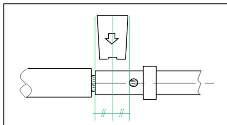
The indent must be placed between the edge of the crimp barrel and the end of the sight hole. The optimal positioning is centered between the edge of the crimp barrel and the beginning of the sight hole.
