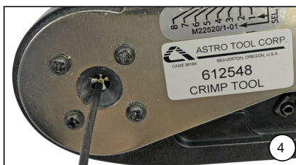
(iii. 3) Insert the crimping sleeve into the pliers. Close until fixed.
