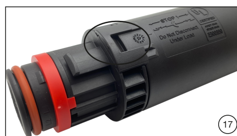
(ill. 16 - 17) Align the snap fit and snap fit receivers of the rear insulation and front insulation. Then slide the rear connector insulation onto the front connector insulation until the snap fits are fully engaged (click sound).
