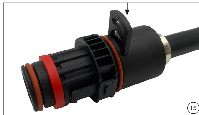
(ill. 14 - 15) Insert the crimped metal contact fully into the front connector insulation. Secure the contact in place by inserting the retention clip into the slit located on top of the connector. It needs to be fully engaged and flush with the insulator surface.
