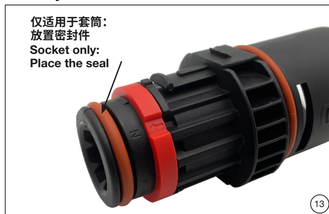
(ill. 12 - 13) Line the arrow on the colored coding ring up with the desired coding position. Slide the coding ring onto front part of the connector insulation. After correct installation the arrow will point toward the desired coding marking. Mechanical coding positions available are PE, +, -, N, L1, L2 and L3. For more information and color options of the ring see page 10. For socket only: Then slide the sealing ring into place.
