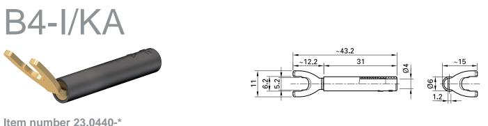
Made of brass for permanent installation, e.g. for connecting screw terminals. Ø 4 mm rigid socket in insulator accepting spring-loaded Ø 4 mm plugs with rigid insulating sleeve. Fork lug bent to an angle of 45°.
