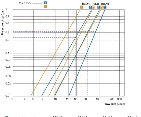
Test conditions: Test fluid: water - density: 998 kg/m<sup>3</sup> - viscosity: 1.08 cSt Direction of flow: Socket → Plug
